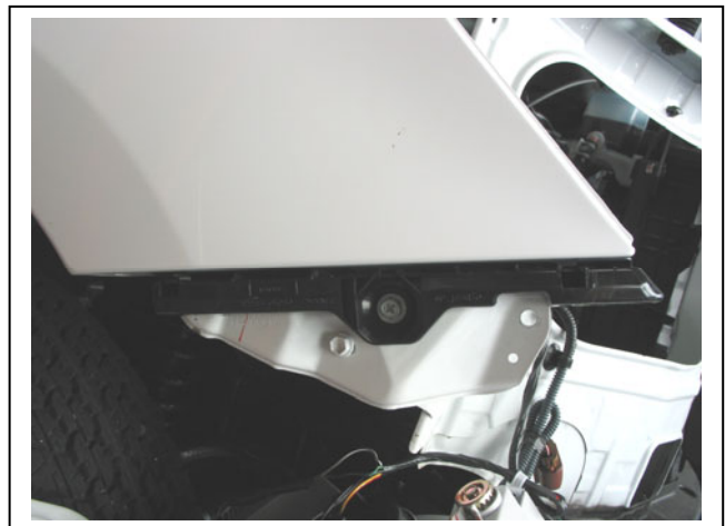
Figure 6 - Remove plastic bumper support from under guard.
