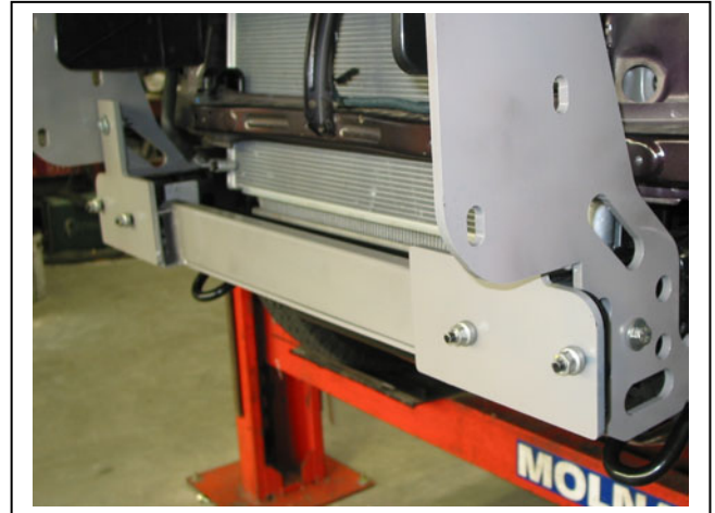
Figure 10 – Steel mounts fitted
