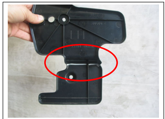
Figure 2: Trim lower section from air dam. Passengers side shown.
