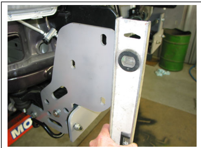
Figure 11 - Passenger side shown Levelling off front edge
